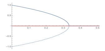
• d = 1: there exists a bifurcation point  $D = D_*$  such that the only stationary solution corresponds to  $\mathbf{u}_f = 0$  if  $D > D_*$  and there are three solutions corresponding to  $\mathbf{u}_f = 0, \pm u(D)$  if  $D < D_*$ **Q**  $\mathbf{u}_f = 0$  is linearly unstable if  $D < D_*$
