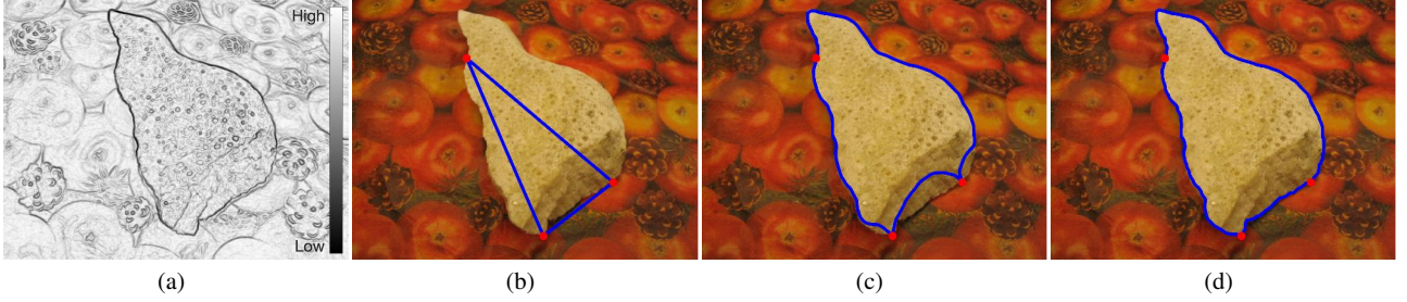
Fig. 12 Image Segmentation results with respect to different tensor fields \mathcal{M} . a The visualization for the eigenvalues \tilde{\lambda}_1 of \mathcal{M} . b Initialization contour generated by the polygon construction method. The landmark points are indicated by red dots. c Image segmentation using \mathcal{M} associated with weights \ell_{\text{mag}} = \ell_{\text{aniso}} = 0 . d Image segmentation using \mathcal{M} associated with weights \ell_{\text{mag}} = 2 and \ell_{\text{aniso}} = 1 .
