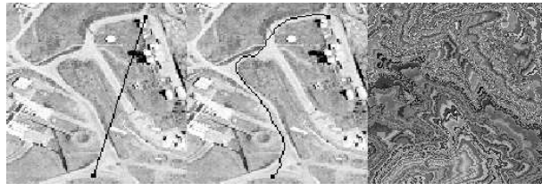
FIGURE 3. Global minimum of active contour model. After giving two points on the left, the minimal path between them is found in the middle image. On the right we show the cost function from the start point. Notice faster propagation along the roads. Potential is defined as a decreasing function of the gray level.
