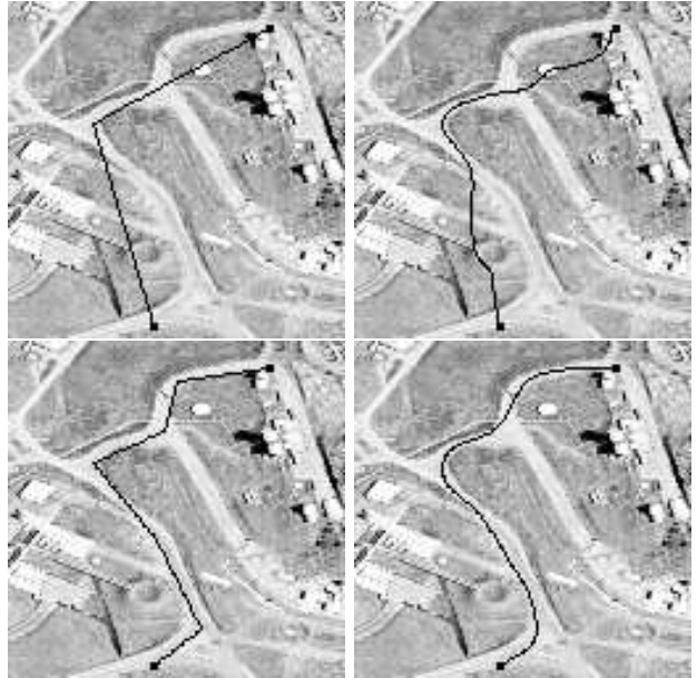
Figure 1: Local Minimum. The initial data is shown on the left and the result on the right. Results of two different initializations of the classical snakes.
