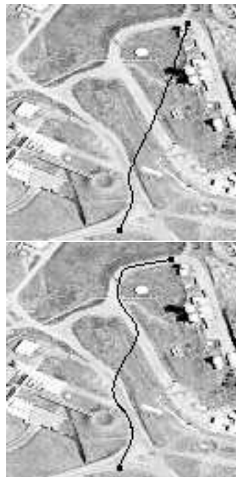
Fig. 10. Two examples of applying the approach of (Neuenschwander et al. 1994) with two slightly different initializations. In both cases the curve is trapped by a local minimum (see text).
