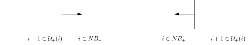
Figure 1: Representation of the useful points and of the Narrow Band for the control \alpha = + . Left: f_+(x_i) > 0 and the discontinuity moves to the right. Right: f_+(x_i) < 0 and the discontinuity moves to the left.
