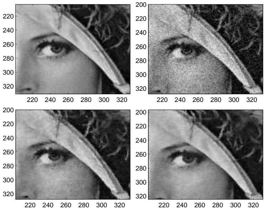
Figure 3: Top: zoom of the original (left) and noisy (right) images, down: zoom of the restored images using the non linear diffusion method (left) and the topological gradient method (right).
