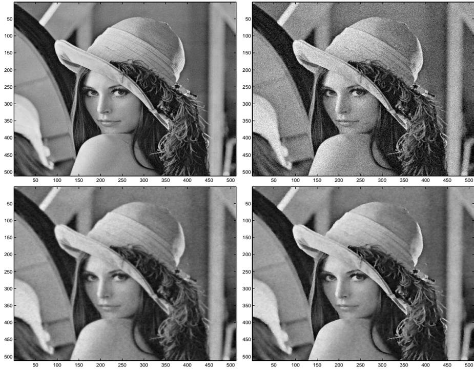
Figure 2: Top left: initial Lena image ( $512 \times 512$  pixels), top right: noisy image (SNR=17), down left: restored image using an homogeneous diffusion method (SNR=27), down right: restored image using topological gradient method (SNR=29).
