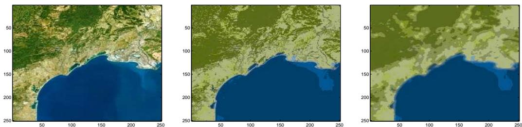
Figure 13: Original image (left), classified image without regularization (center), and regularized and classified image (right).
