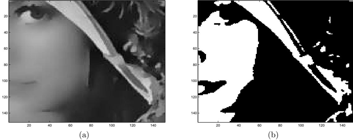
Figure 11: Two-classes classified image obtained using the topological gradient algorithm applied to the new equation for smoothing (a) and then the closest class algorithm for classification (b).
