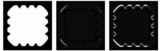
Fig. 8. Curvature metric. Left: original slice of the 3D image. Center and right: curvature of the contours in the principal directions represented as \mu_2 and \mu_3 , respectively.
