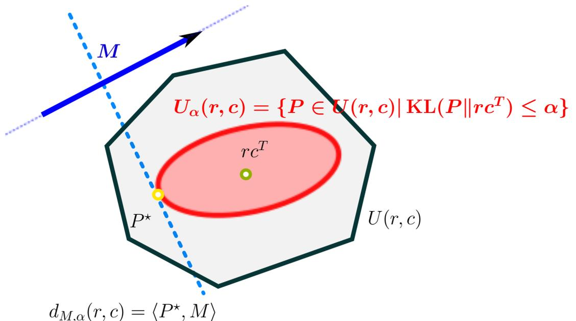
FIGURE 1. Schematic view of the transportation polytope and the Kullback-Leibler ball of level  $\alpha$  that surrounds the independence table  $rc^T$ . The Sinkhorn distance is the dot product of  $M$  with the optimal transportation table in that ball.
