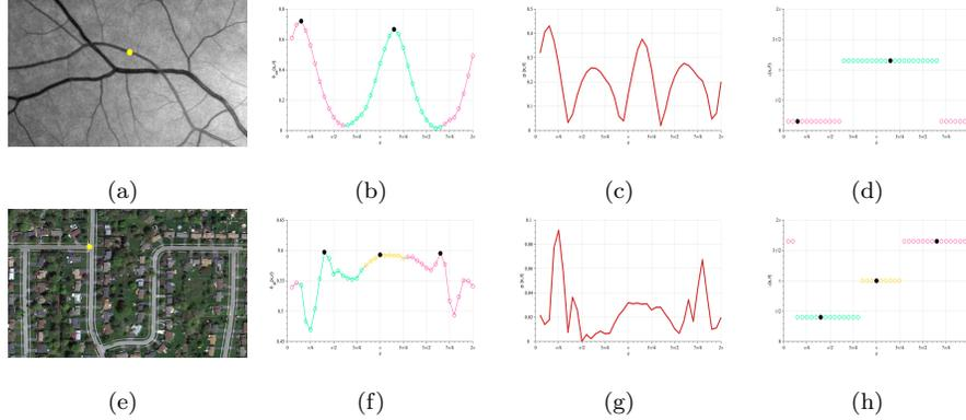
Figure 2: Examples for coherence-enhancement appearance features and orientation clustering. (a) and (e) Retinal and road images patches with points denoted as yellow dots. (b) The coherence-enhanced orientation score. (f) The multi-orientation coherence enhancing gray level score. (c) and (g) Values of the potential maps associated to the yellow points. (d) and (h) The clustered orientations.
