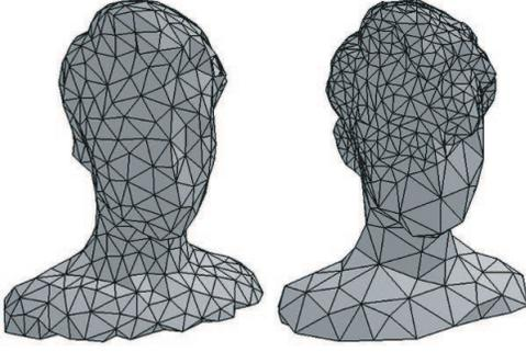
Figure 11. Uniform (left) and user-defined remeshing (right).
