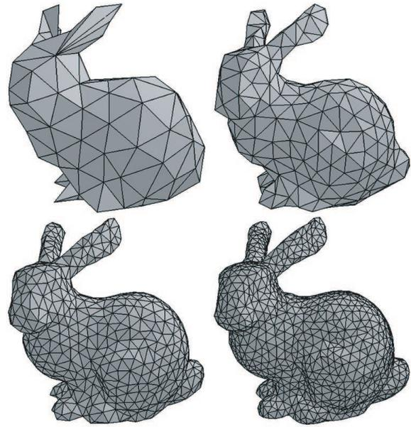
**Figure 9. Geodesic remeshing with 100, 300, 800 and 1500 points.**
