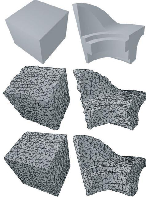
Figure 14. Original model (top), uniform remeshing (middle) and curvature-based remeshing (bottom).
