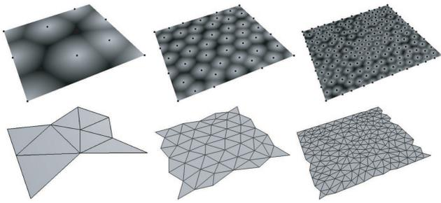
**Figure 8. Insertion of points in a square (top), and corresponding triangulation (bottom).**
