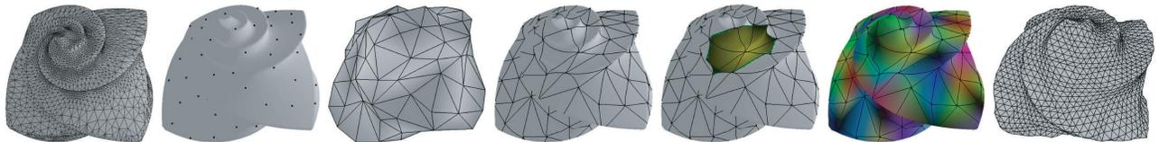
Figure 1. Different steps in mesh parameterization.
