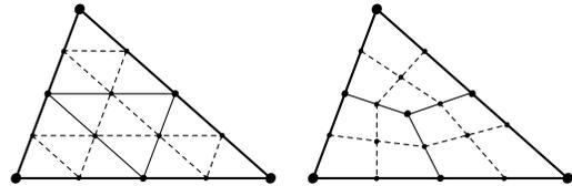
**Figure 19. Triangle-based and quad-based subdivision schemes.**
