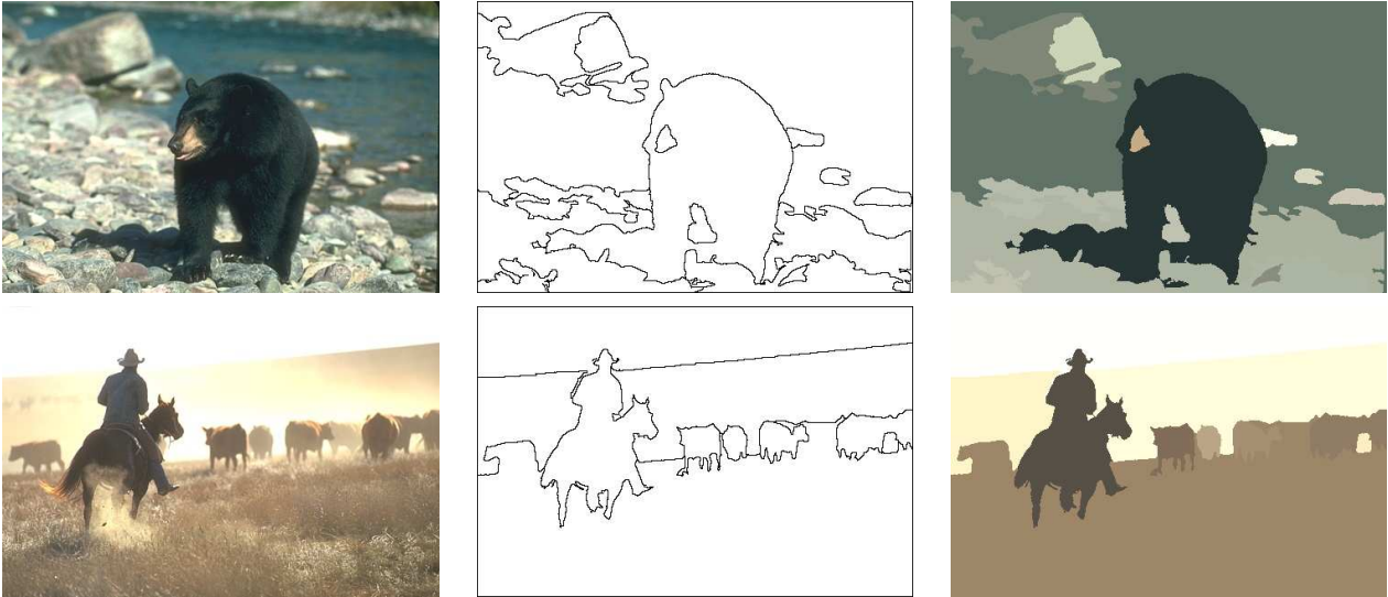
Figure 5: From left to right: original images, tessellations and mosaic images with median color. Top: 15 zones and \alpha = 0.23 . Bottom: 10 zones and \alpha = 0.3 .
