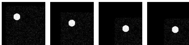
Figure 9: Registration with Gaussian additive noise. From left to right the four first iterations of the process at scale 1. We come up with a translation parameter of (99.66,100.07).
