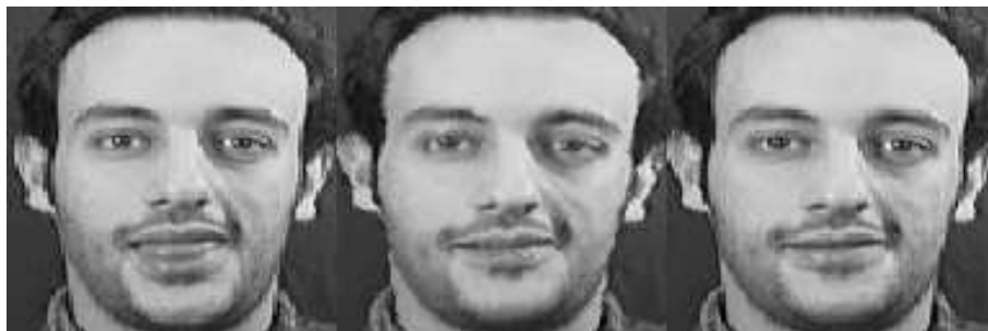
Figure 20: Registration of a face with two different expressions: Study image (left), deformed Study image onto Target image (center), and Target image (right).
