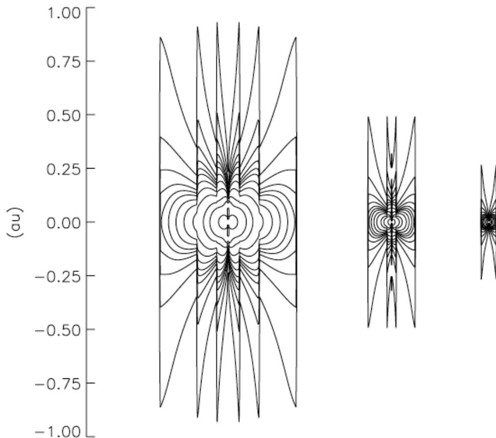
Figure 2: Contour plots of iron atoms in DM theory in magnetic fields  $B = 10^8$ ,  $10^9$  and  $10^{10}$  T
