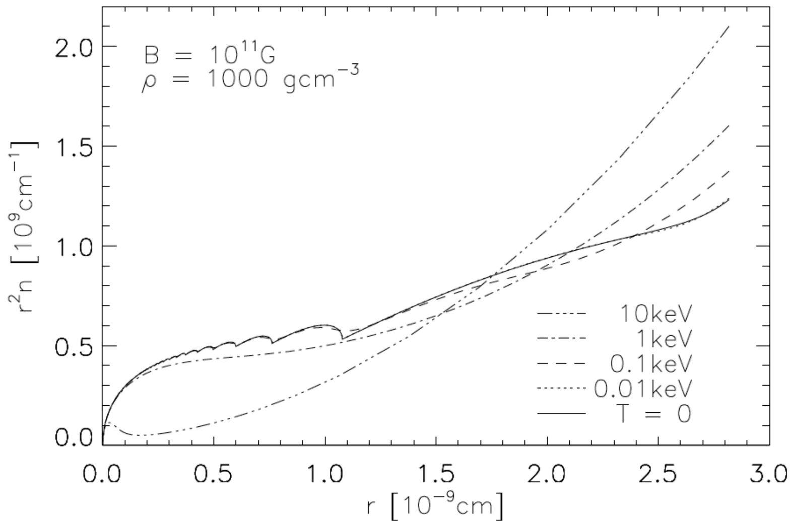
Fig. 3.— The quantity  $r^2 n$  for a spherical unit cell of iron in the TF approximation. The matter
